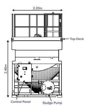
Additional extras (sludge pump, rake, top deck and controller) hired under separate rates under combined package.
