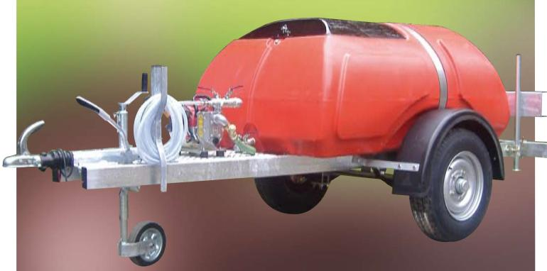
THIS 1100 LITHE PLASTIC WATER BOWSER COMES COMPLETE WITH A BOOMINATOR SPRAYING SYSTEM, 1" HONDA PETROL PUMP, AND SPRAY GUN. IDEAL FOR WATERING THE GREENS, DAMPING DOWN QUARRIES, RACECOURSES ETC AND IN ANY SITUATION WHERE DUST SUPPRESSION OR WATERING IS REQUIRED.
