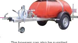
The bowsers can also be supplied as a 'site' model. This model is designed specifically for off-road use, and will be fitted with an unbraked axle. No suspension mudguards or brakes will be supplied.
