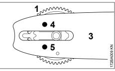
Position the tensioning gear (1) against the guide bar (3) so that the stud (4) projects through the upper hole and the short guide peg (5) locates in the lower hole.
