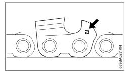
The chain pitch marking (a) is embossed in the area of the depth gauge of each cutter.
