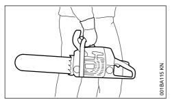
Always carry the chain saw by the handle – with the hot muffler away from your body, the guide bar must point to the rear. To avoid serious burn injuries, avoid touching hot parts of the machine, especially the surface of the muffler.
