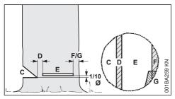
The **felling notch** (C) determines the direction of fall.
