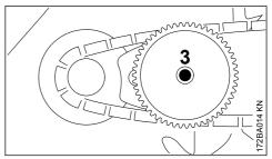
Fit the chain sprocket cover so that the wingnut locates on the collar screw (3).
