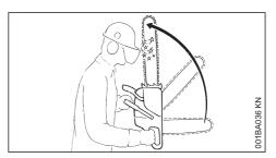
(Kickback) occurs when the saw is suddenly thrown up and back in an uncontrolled arc towards the operator.
