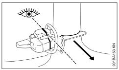
Insert the chainsaw with guide bar in the bottom of the felling notch. The gunning sight must point in the planned direction of fall – if necessary, correct direction of fall by re-cutting the felling notch.
