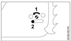
Turn the screw (1) counterclockwise until the tensioner slide (2) butts against the left end of the housing slot.
