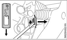
Use the combination wrench or a screwdriver to ease the shutter out of the summer position <sup>1</sup>/<sub>2</sub>.
