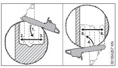
Perform this felling cut when the tree diameter is greater than the cutting length of the chainsaw.
