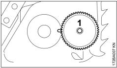
Remove the tensioning gear (1) and turn it over.
