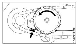
Guide the drive link into the bar groove (see arrow) and turn the tensioning gear to the left as far as possible
