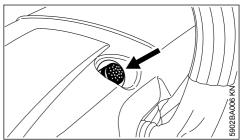
Press the button, the decompression valve will be opened
