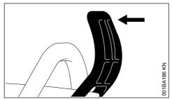
Pull the hand guard towards the front handle until there is an audible click – the chain brake is disengaged. 6.3 Fitting the chain
