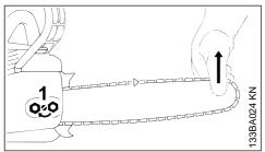
Retensioning during cutting work:
