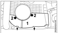
Place the cover plate (1) in position, engage the two tabs (arrows), and secure it with the screws (2).
