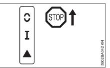
**STOP** or 0 – Master Control lever must be pushed in direction of **STOP** or 0 to switch off ignition. The Master Control lever springs back to the run position I when it is released.
