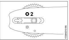
Screw the nut (2) on to the stud as far as stop by hand.
