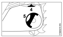
When fitting the chain sprocket cover, the teeth of the adjusting wheel and the tensioning gear must mesh; if necessary,
