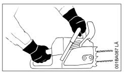
Always hold the chain saw **firmly with both hands:** Right hand on the rear handle – even if you are left-handed. To ensure reliable control, wrap your thumbs tightly around the handlebar and handle.
