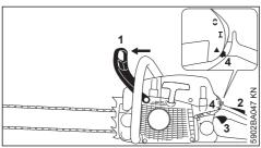
Push the hand guard (1) forward – the chain is locked.
