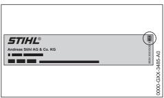
The STIHL M-Tronic version is indicated on the approval label of the chain saw, e.g. "M3.0" indicates the STIHL M-Tronic version 3.0.
