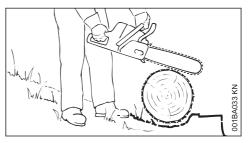
If on a slope, stand on the uphill side of the log. Watch out for rolling logs.
