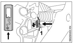
Refit the shutter the other way round in the winter position – the arrow points to the symbol \* – the shutter must snap into position.
