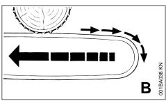
Pushback occurs when the chain on the top of the bar is suddenly pinched, caught or encounters a foreign object in the wood. The reaction of the chain drives the saw straight back toward the operator – **to avoid this risk**:
