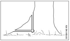
Remove largest buttresses: first the largest buttress – saw first vertically, then horizontally
