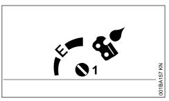
Use the adjusting screw (1) (on underside of machine) to vary the oil feed rate as required.
