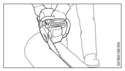
Sawing technique without use of the spiked bumper – risk of pull-in – position the guide bar at as shallow an angle as possible – be especially careful – increased **risk of kickback!**
