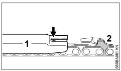
Lay the appropriate file gauge (1) for the chain pitch on the saw chain and press it against the cutter to be checked – if the depth gauge protrudes past the file gauge, the depth gauge must be reworked
