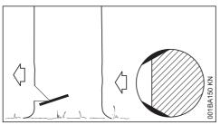
Sapwood cuts in long-fibered softwood help prevent sapwood splintering when the tree falls. Make cuts at both sides of the trunk at same height as bottom of felling notch to a depth of about 1/10 of trunk diameter. On large diameter trees, cut to no more than width of guide bar.
