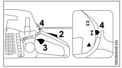
If the engine was started in the start position ▲: Press down trigger lockout (2) and the pull the throttle trigger (3) at the same time – the Master Control lever (4) moves to the run position I and the engine settles down to idling speed.
