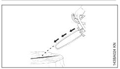
The saw chain must always spin off a small amount of oil.
