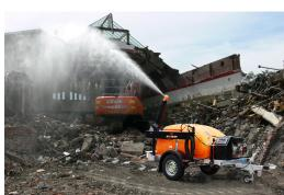
The JETMISTER is a revolutionary dust suppression bowser that will solve most construction and demolition site dust issues. 2000 Ltr (440 G) Water bowser that can easily be positioned to tackle the dust. 10 to 30 metre throw powered by either a diesel engine or an electric pressure pump with a 45° or 90° auto oscillating jet nozzle on a tilting mast.
